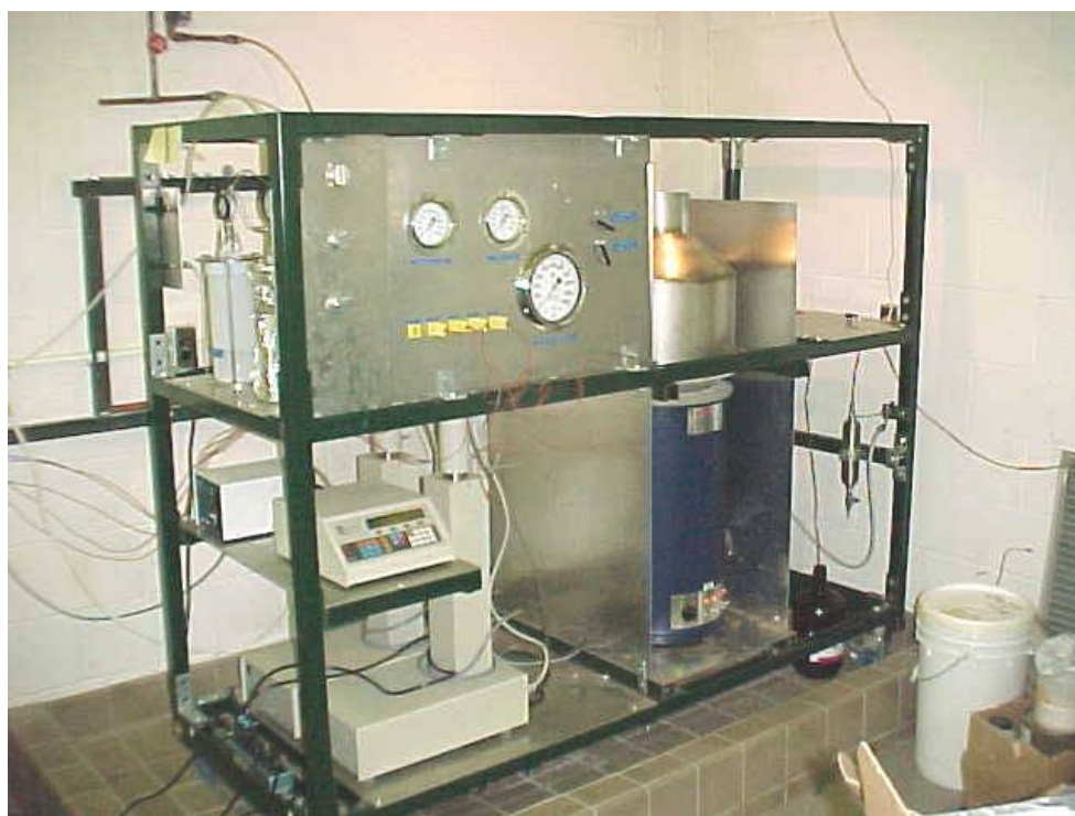
Figure 16. Supercritical Water Oxidation apparatus at Clemson University
