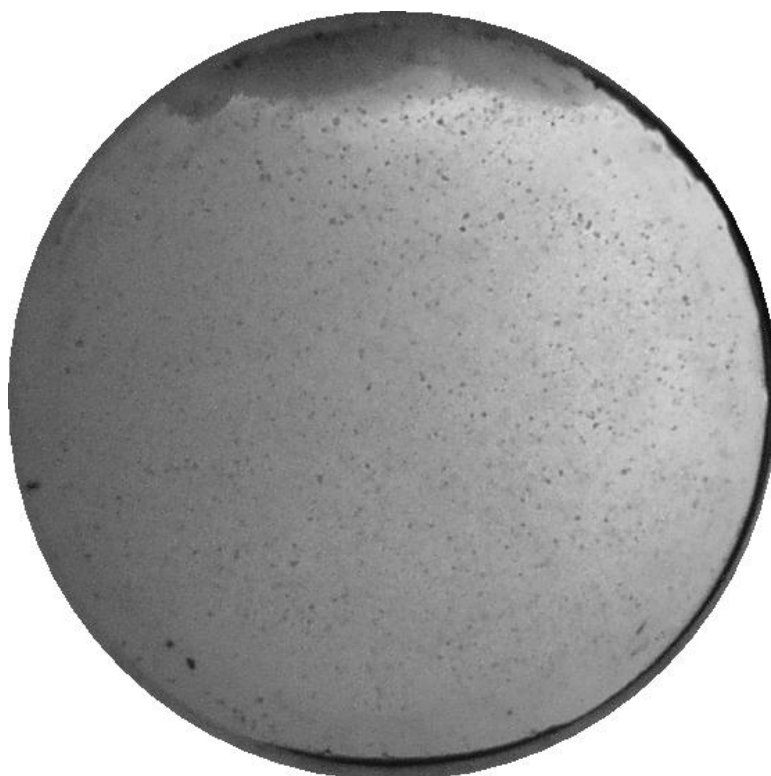
FIGURE 7. CO 2 -in-Water Emulsion Stabilized by CaCO 3 Particles in the Presence of MEA.
