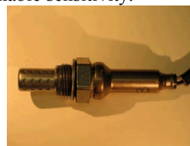
Figure 9. Photograph of Pt/YSZ/Au prototype built on a heated substrate and packaged into an oxygen sensor housing.
