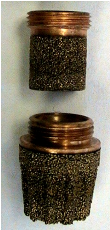
Figure 10 Nozzle (double) filter, fairly clean, with 1405 hours on-time
