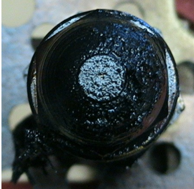
Figure 9 Fouled nozzle tip, after 1405 hours of on-time operation
