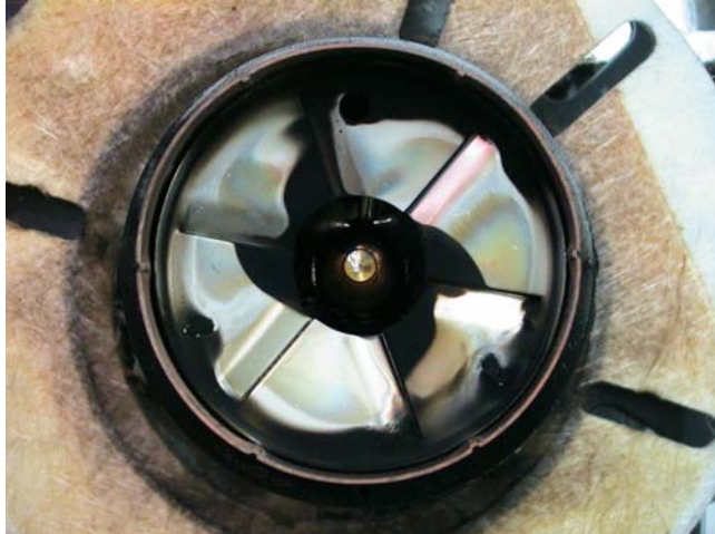
Figure 5 Combustion head and nozzle
