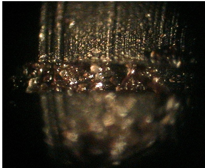
Figure 128 Slot partially blocked by fuel “varnish”
