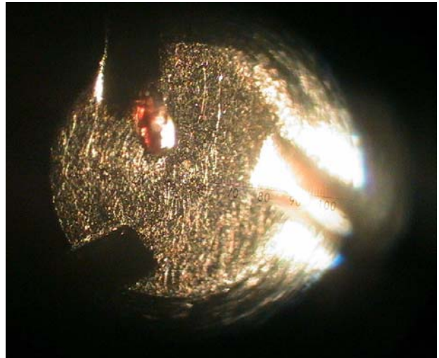
Figure 8 Top of fuel distributor cone, 3 slots
