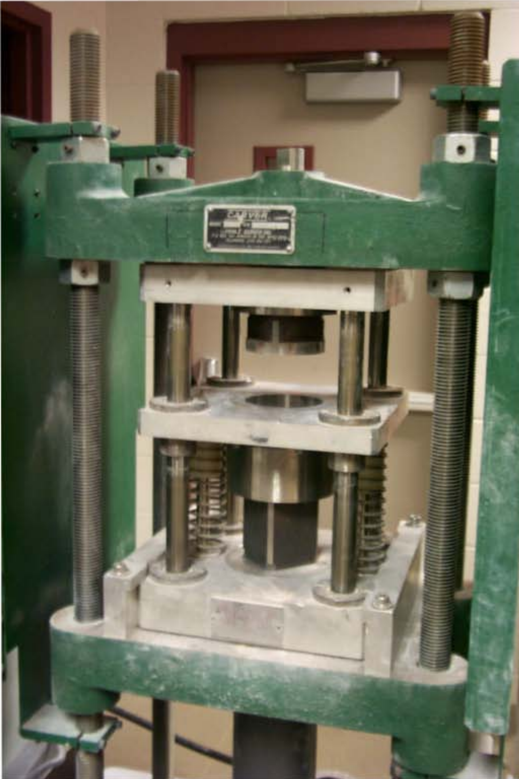
Figure 3: Double-action die assembly mounted in 30-ton press.
