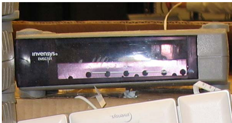
Figure 2.3. Invensys Controls GoodWatts Home Gateway
