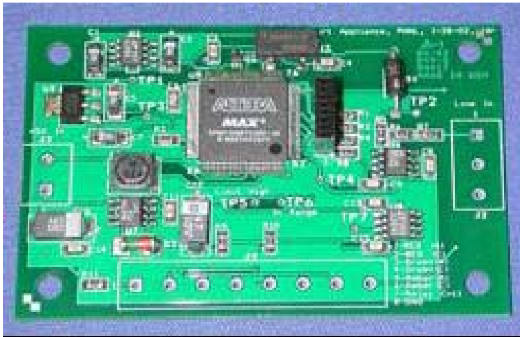
Figure 1.3. GFA Controller Board used in the Grid Friendly Appliance Project
