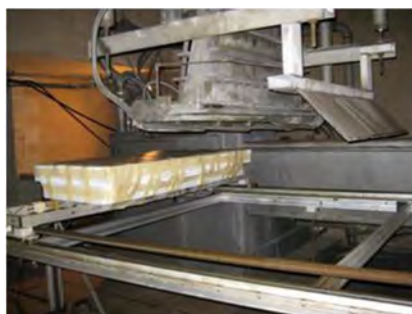
Figure 8. Electron Beam Set-up Used For Irradiating Braids and Leno Woven Fabrics
