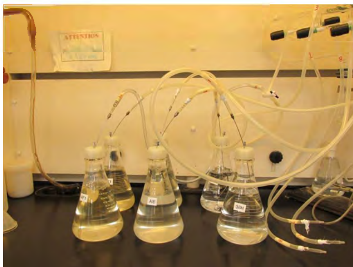
Figure 12. Degassing Graft Solutions
