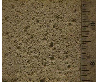
Figure 2.4. Concrete Membrane Surface with Extensive Air Bubble Imprints (Batch #2, Mold II Specimen)
