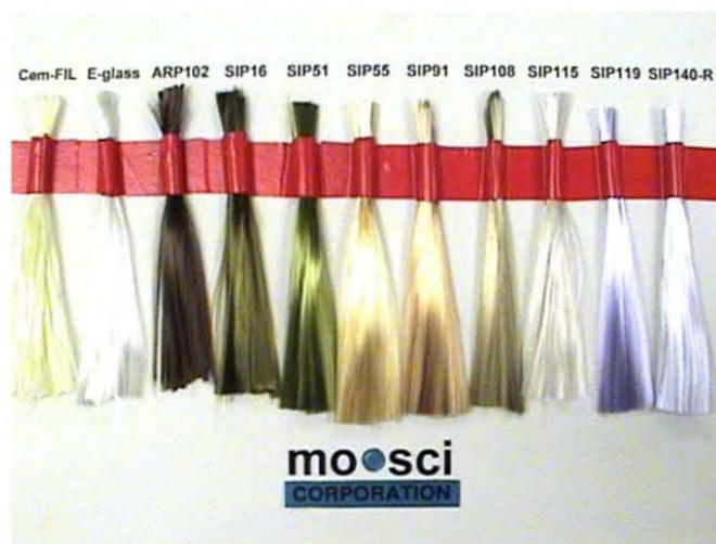
Figure 2. Samples of continuous Ca-Fe-phosphate fibers manufactured at MO-SCI Corp. The color is dependent upon the glass composition. The commercial silicate glasses CemFIL ® and E-glass, are shown on the left.
