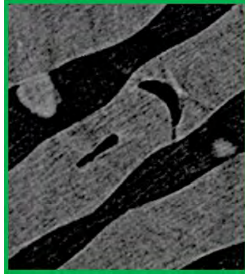
Figure 17: Internal porosity
