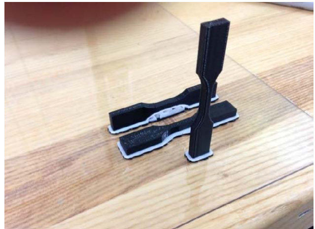
Figure 7: X, Y and Z type V dogbones
