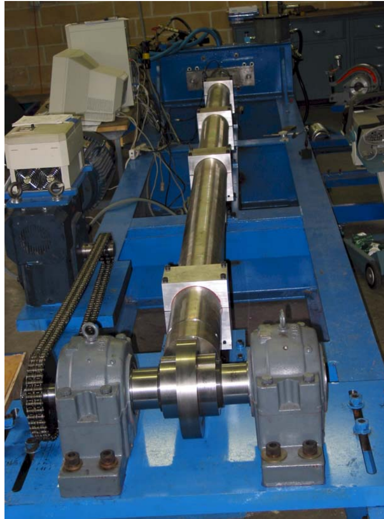
Figure 10: DVMCS laboratory prototype under testing on test bench
