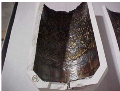
Figure 10. Cross sectional view of a dense high silica crucible after 14 days at 1250°C with the iron phosphate melt containing 27 wt% LAW (IP27LAW).
