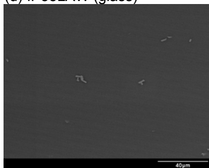
Figure 2. SEM micrographs and XRD patterns of iron phosphate glasses containing 27, 32, and 35 wt% LAW (IP27LAW, IP32LAW, and IP35LAW, respectively).
