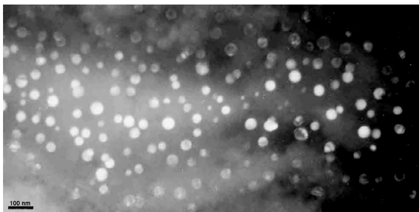
Figure 5. Dark-field TEM photo of the Ni 3 Si precipitates in the specimen aged for 24 h under an applied stress of 50 MPa.
