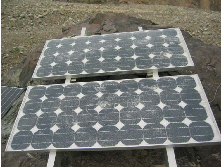
Damaged solar cells at Al Hayl station
