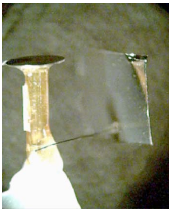
Target for the collapsing radiative shock experiments built at Michigan.
