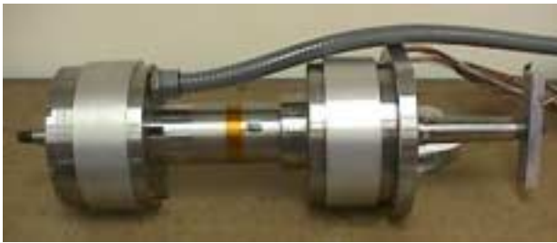
Figure 9. Magnetic rotor/bearing system for grinder
