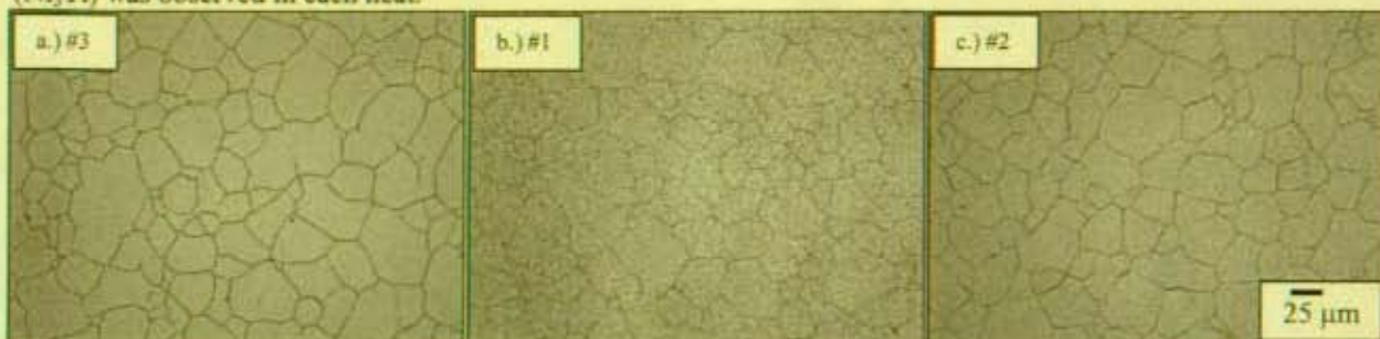
Figure 2. Comparison of the grain structure of the heats of X-750 AH investigated in this study. Electrolytically etched in 8:1 phosphoric acid in water, 3V.
