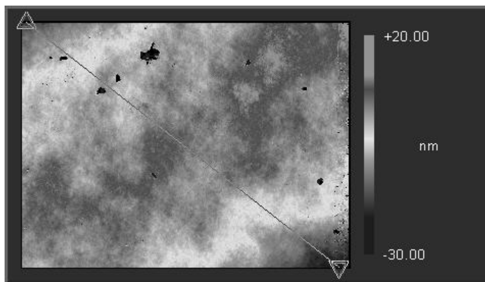
Fig.16. The surface profile taken at another location on the SiC chip and its corresponding cross-section is shown in Fig.17.
