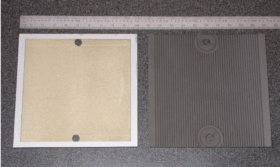
Figure 24 Interconnects fabricated for SORFC stack testing
