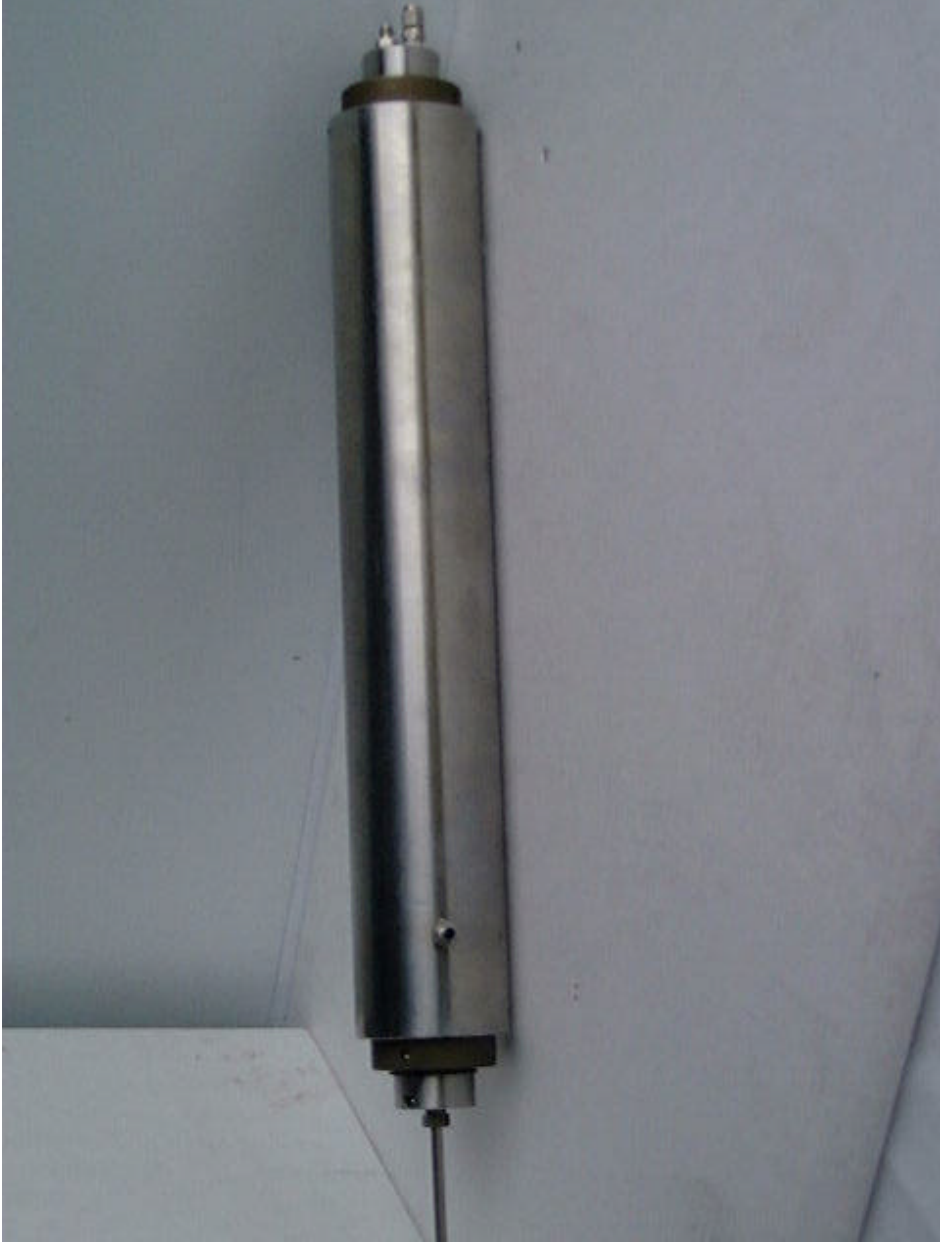
Fig. 1a - Temco core holder used for high temperature treatment
