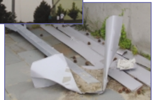
Figure 19. The Evans Residence turbine fell after a guy wire failed. Here you see the tail crushed with embedded rocks and soil. Next to it lay the blades.
