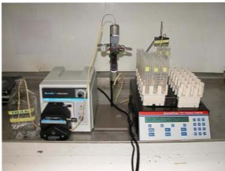
Fig. 3. Experimental setup for ion exchange tests.
