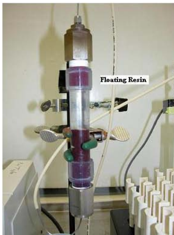
Fig. 6. Floating resin at start of loading cycle.
