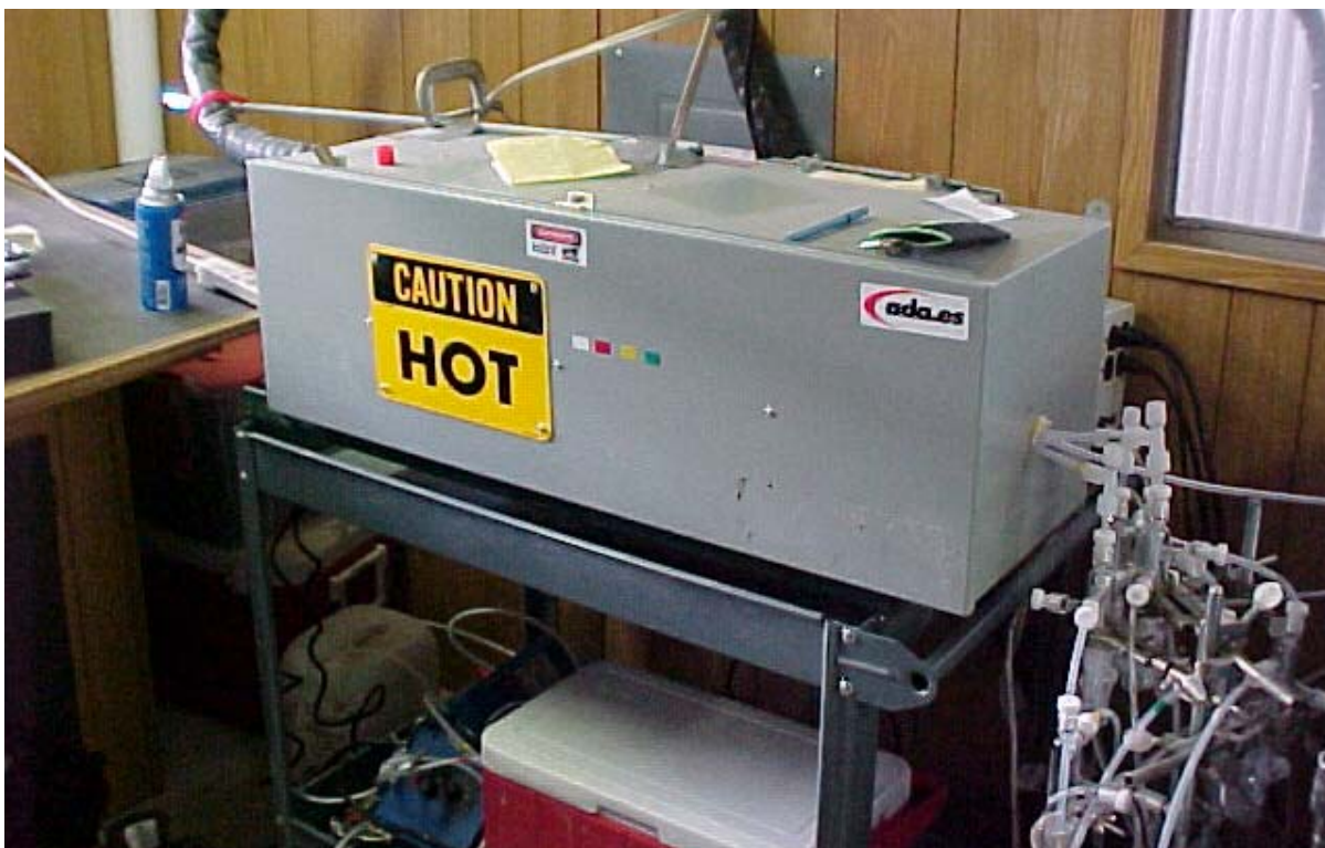
Figure 5. Sorbent Screening Device—Heated Box and Impingers.
