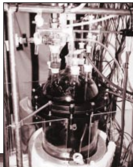
40-liter glass Acid Digestion pilot-scale reactor
