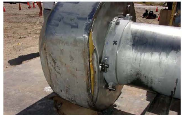
Figure 9. Deformed Shape of Lid-End Impact Limiter After a 30-Foot Drop Test
