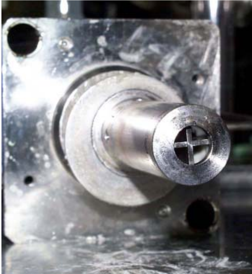
Fig. C-2. White Solids Plugging the Rotor in Stage 15
