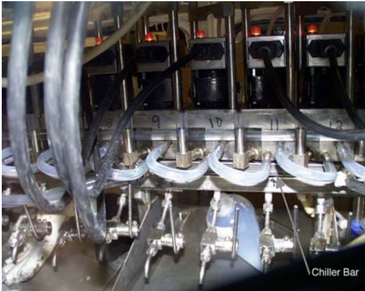
Fig. A-2. Location of Chiller Bars on 2-cm Contactor
