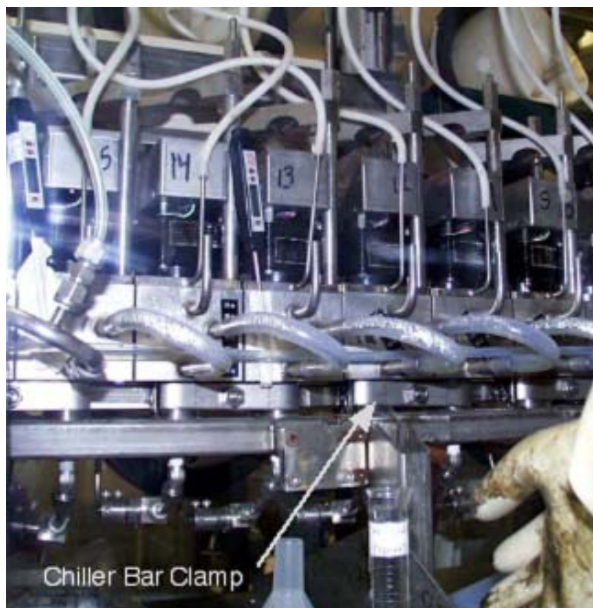
Fig. A-4. Clamps for Chiller Bars
