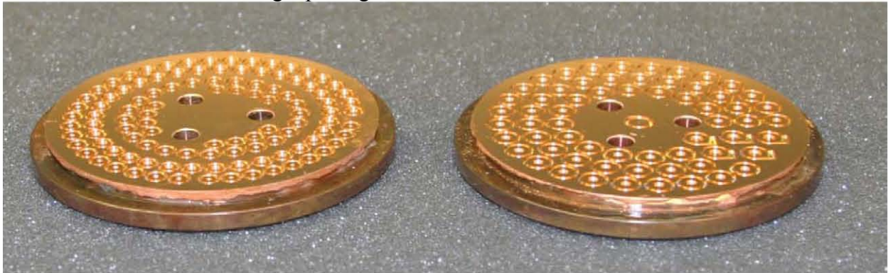
Figure 12. Mandrels that have been milled with patterns of support rings
