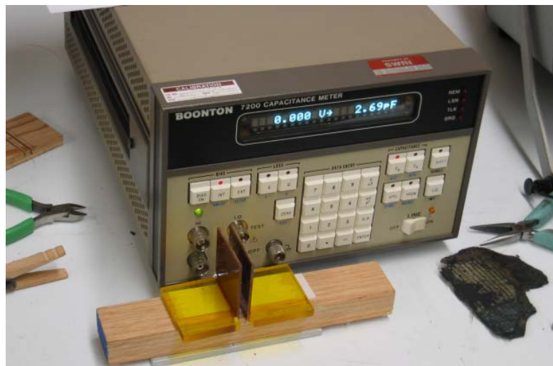
Figure 5. Setup for measuring dielectric constant of pipe coating
