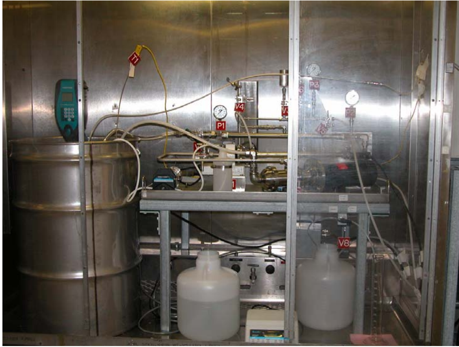
Figure 2. Crossflow Filter Unit
