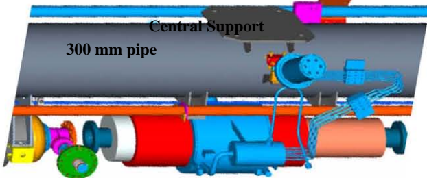
Current leads Quadrupole and Corrector Package SCRF
