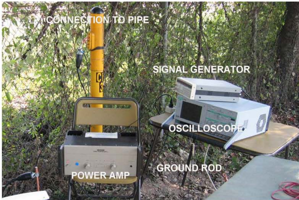
Figure 6. Instrumentation setup near CP3
