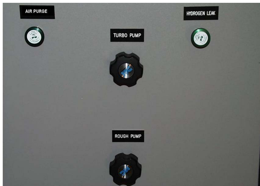
Figure 2.6. Location of Vacuum Control Valve Handles on Outside of Main Cabinet (One Set on Each Side for Each Test Chamber).
