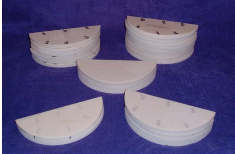
Figure 1. The BRTES phantom series of varying glandularity and compressed breast thickness.
