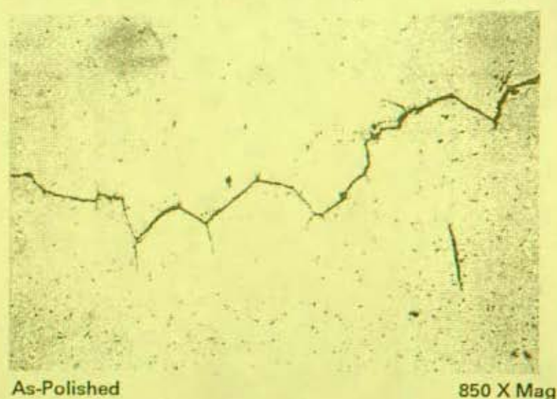
FIGURE 5 - IGSCC Crack Paths in Grade 8 Steel Exposed to Boiling Ammonium Nitrate
