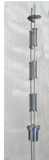
Figure 4 DEOX Off-Gas Trapping System
