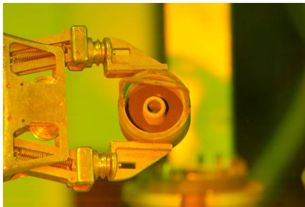
Figure 13 A close-up view of the Inconel crucible with powdered fuel created during DEOX processing.
