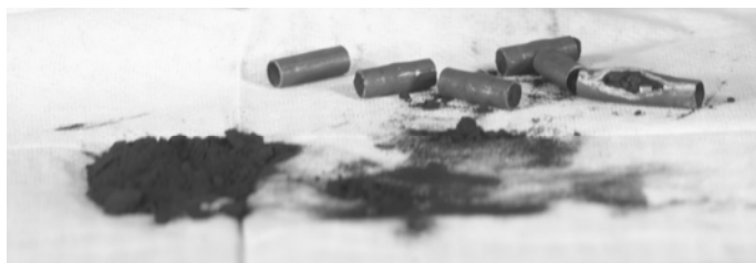
Figure 1 Spent fuel after voloxidation experiment
