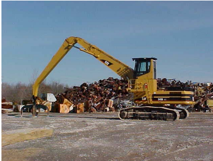
Figure 3a. Caterpillar Material Handler with Rotating Grappler
