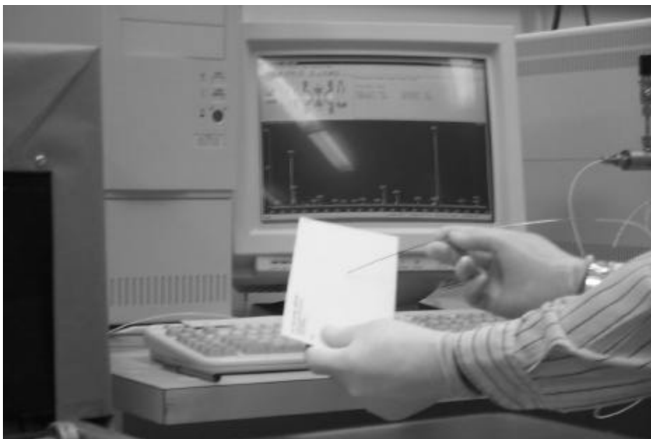
Figure 8: Detection of a PFDMCH ( m/z = 400 ) marked envelope by DSITMS.
