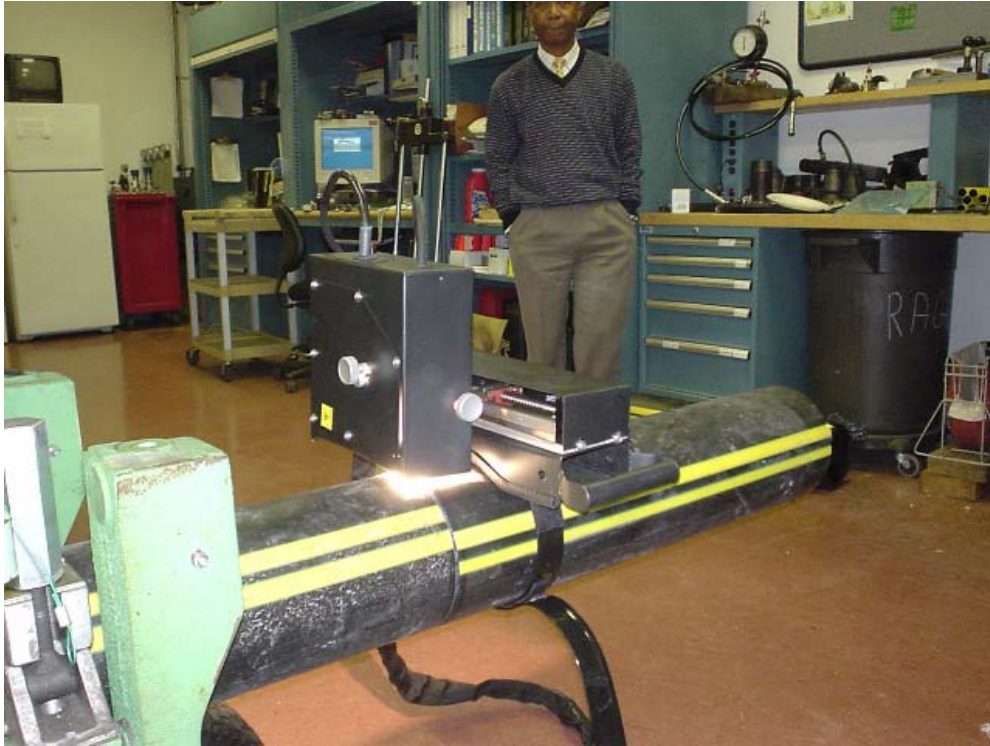
Figure 14 Inspection System on Pipe during Heating Phase of Inspection Process
