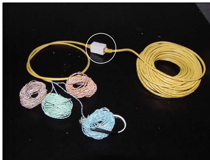
Figure 4: Data acquisition wiring assembly
