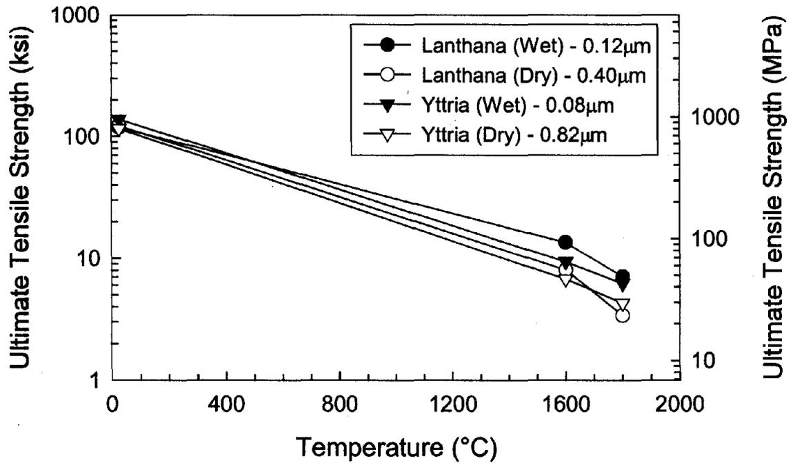
Figure 1. The effect of oxide species and processing method on the strength of 2 vol.% ODS molybdenum material as a function of temperature.
