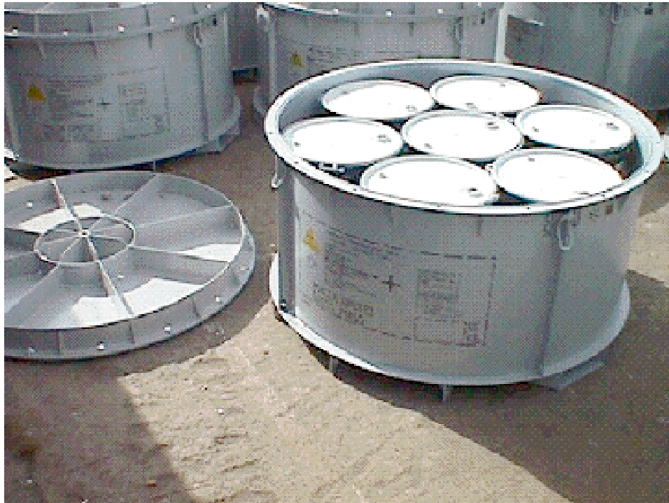
Fig. 2. PST1A-6 Container with Seven Standard 200-liter Drums
