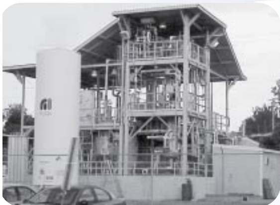
The University of South Carolina's Filtration Research Engineering Demonstration facility was used to demonstrate crossflow filtration in the alpha and strontium removal process.
