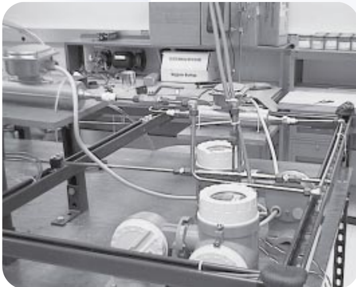
Dual Coriolis density meters in the FIU test loop.
