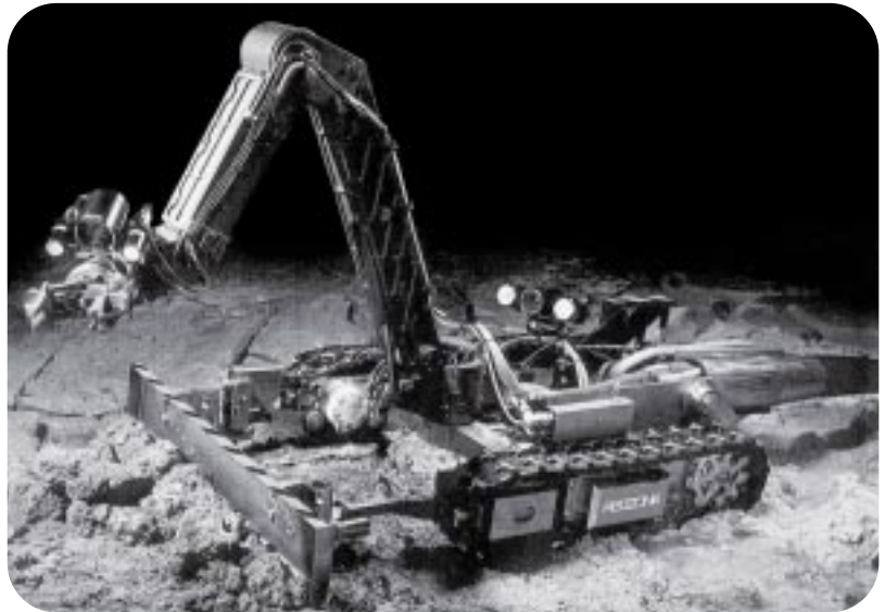
By integrating the Confined Sluicing End Effector with the remote capabilities of the Modified Light Duty Utility Arm and the Houdini vehicle (pictured here), TFA helped deliver a highly successful method for retrieving waste from the gunite tanks.
