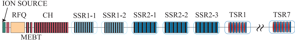
Figure 1: Schematic layout of the front-end of the FNAL 8-GeV superconducting linac.
