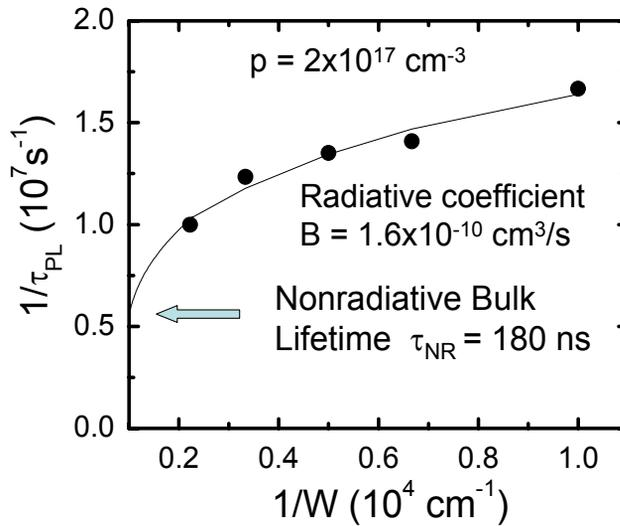
Having photon recycling factor  $\phi$  calculated, lifetime data for 0.54 eV GaInAsSb were fitted by  $1/\tau_{\text{NR}} + B\rho/\phi(W)$ , using nonradiative bulk lifetime  $\tau_{\text{NR}}$  and radiative coefficient  $B$  as parameters. The best fit was achieved with  $\tau_{\text{NR}} = 180 \text{ ns}$  and  $B = 1.6 \times 10^{-10} \text{ cm}^3/\text{s}$ .
