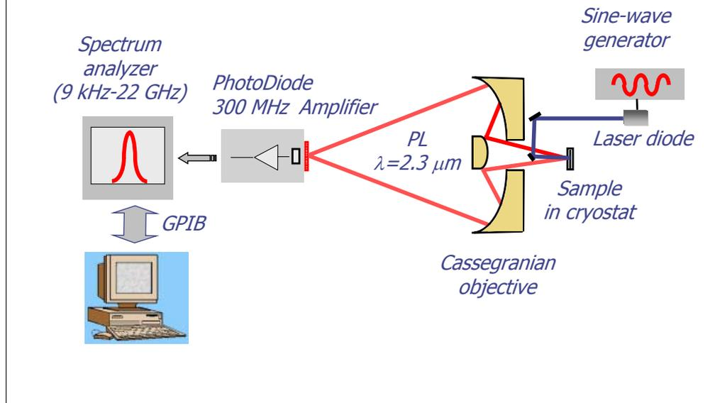
The figure shows schematic of the experimental setup for optical response measurements. Excitation source is AC modulated laser diode operating at 1.3  $\mu\text{m}$ . PL emission of the sample at  $\lambda = 2.3 \mu\text{m}$  was collected by Cassegranian reflective optics and focused to small-area IR photodiode followed by 300 MHz preamplifier. Modulation PL response was recorded by a spectrum analyzer.
