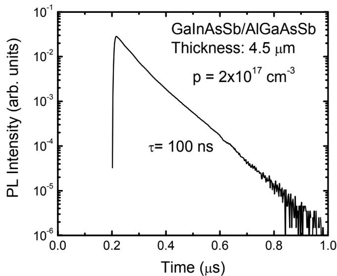
The figure shows typical transient photoluminescence response measured in 4.5- $\mu\text{m}$ -thick AlGaAsSb/GaInAsSb/AlGaAsSb structure. The PL intensity was recorded within several orders of minority carrier concentration which is critical for reliable lifetime determination. Dynamic lifetime of 100 ns obtained by TRPL corresponds to static lifetime measured by optical response.
