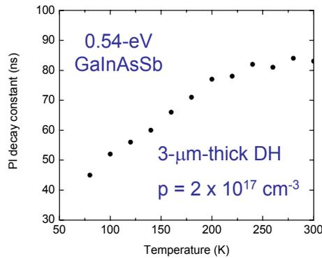
In structures where radiative recombination dominates, total recombination rate should decrease with T. The graph shows lifetime data for 3-um-thick AlGaAsSb/GaInAsSb/AlGaAsSb DH with  $p=2 \times 10^{17} \text{ 1/cm}^3$  measured in the temperature range from 80 to 300 K. Increase of PL decay time with temperature indicated significant role of radiative recombination.
