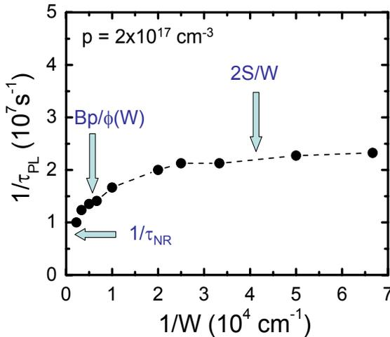
Using wide range of GaInAsSb layer thickness interface and radiative recombination effects can be separated
