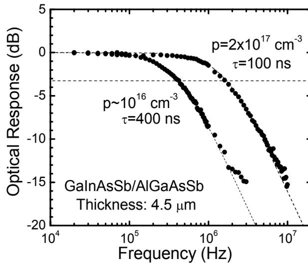
The graph presents optical responses measured in 4.5- $\mu\text{m}$ -thick AlGaAsSb/GalnAsSb/AlGaAsSb undoped and doped samples. PL signal in dB is plotted versus excitation source modulation frequency. -3 dB point corresponds to the frequency of 1.6 MHz which gives recombination lifetime value of 100 ns for the doped structure and 400 ns for the undoped one.
