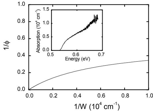
Photon recycling factor for 0.54-eV GaInAsSb DH was calculated using approach similar to that reported by Asbeck (JAP, 1977). This model does not take into account effect of multiple reflection propagation of photons, which is a reasonable approximation for samples with
