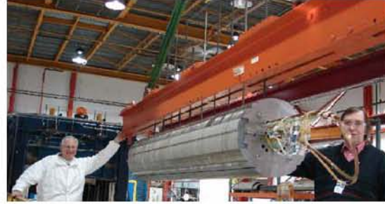
Figure 7: 2-m long mirror LM01 with PIT coil.
