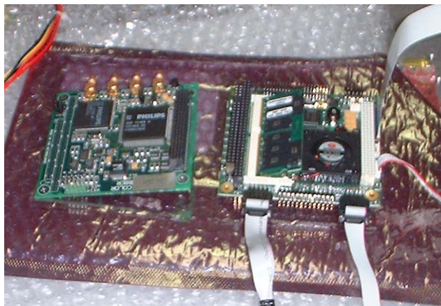
Figure 1. Photos of a board-level computer (left) and a pc/104 computer system (right). Both of these systems will decrease the footprint of the machine vision system and make it easier to utilize the technology in harsh environments.
