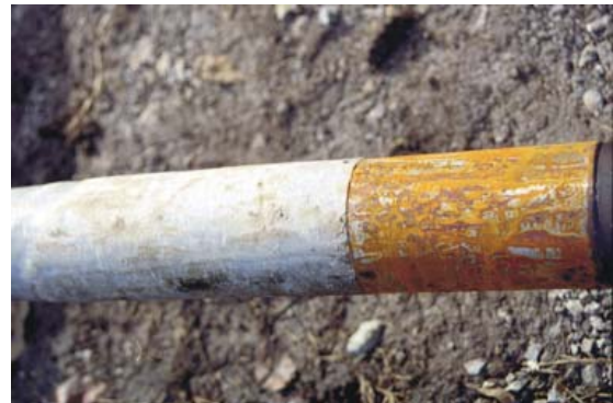
Condition of joint end after use a little rust on the steel end, but the composite has only a few scratches.
