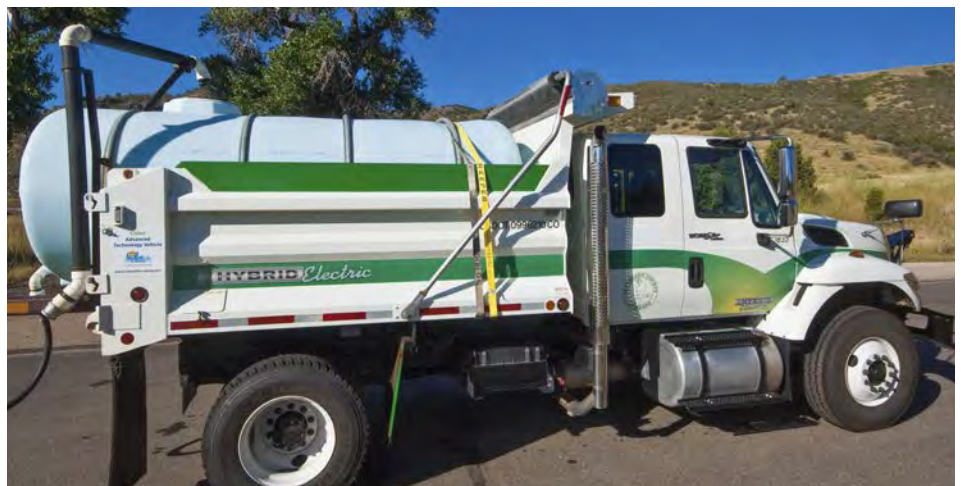
HEVs work well for both light-duty and heavy-duty applications, particularly those that require frequent stops and starts. Photo by Pat Corkery, NREL 18142
