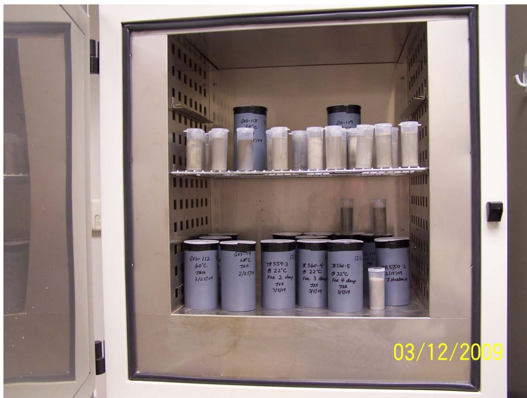
Figure 2-1 Photograph of one of the ovens used to cure the samples at elevated temperatures
