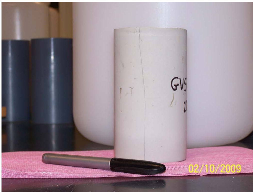
Figure 3-18 Photo of GVS 91 after 90 days of curing showing the longitudinal crack the entire length of the 6 inch long cylinder
