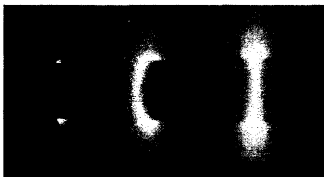
FIGURE 3. Discharge characteristics of DC magnetron sputtering in SNS ring halfcell chamber.
